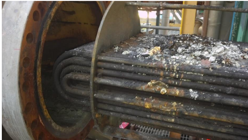
Figure 28 - Fouling on third reheater tubes
