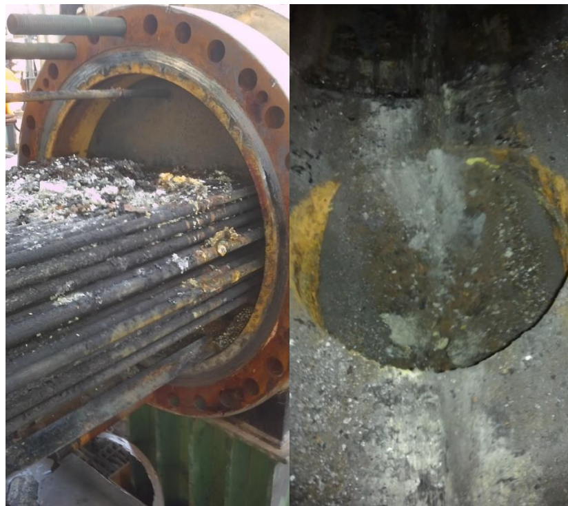
Figure 29 - Fouling on third reheater tubes/fouling in inlet nozzle third reheater
