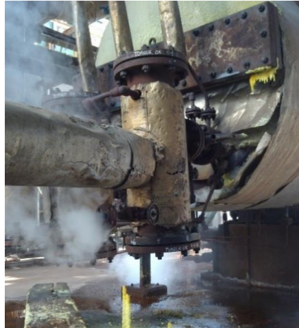
Figure 11 - Sulfur Boot on Third Condenser
