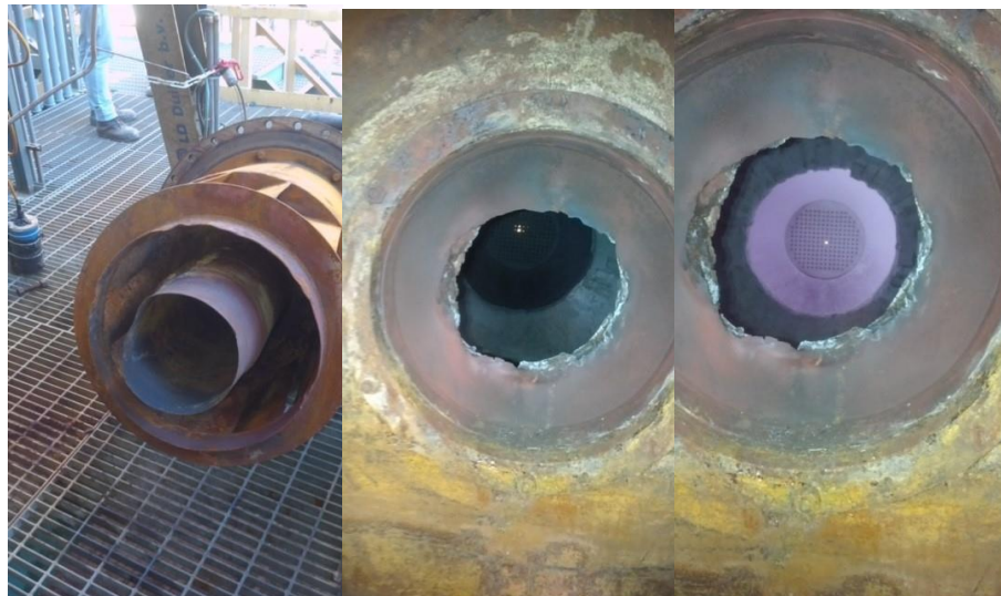
Figure 22 - Main Burner and nose cone into the Mixing Chamber
