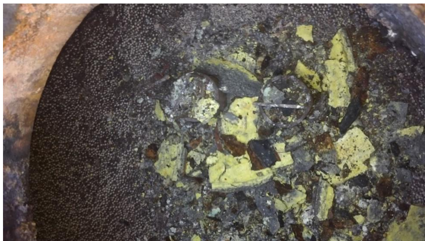
Figure 33 - Top View Catalyst Third Reactor
