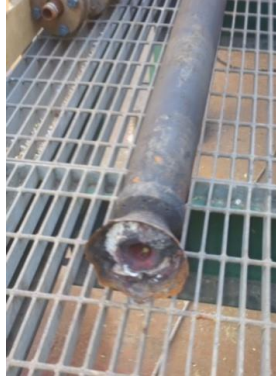
Figure 21 - Natural Gas Gun and Nose Cone Damage
